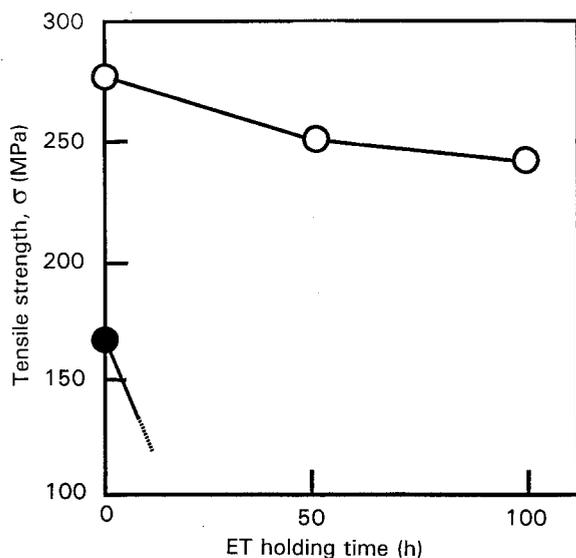
Figure 11 Changes in the (●) SiC/Al-3.0%Mg and (○) ZrC/Al-3.0%Mg (SiC (3.0 μm), ZrC (2.4 μm) composite strengths with the elevated-temperature holding time, at 803 K.
