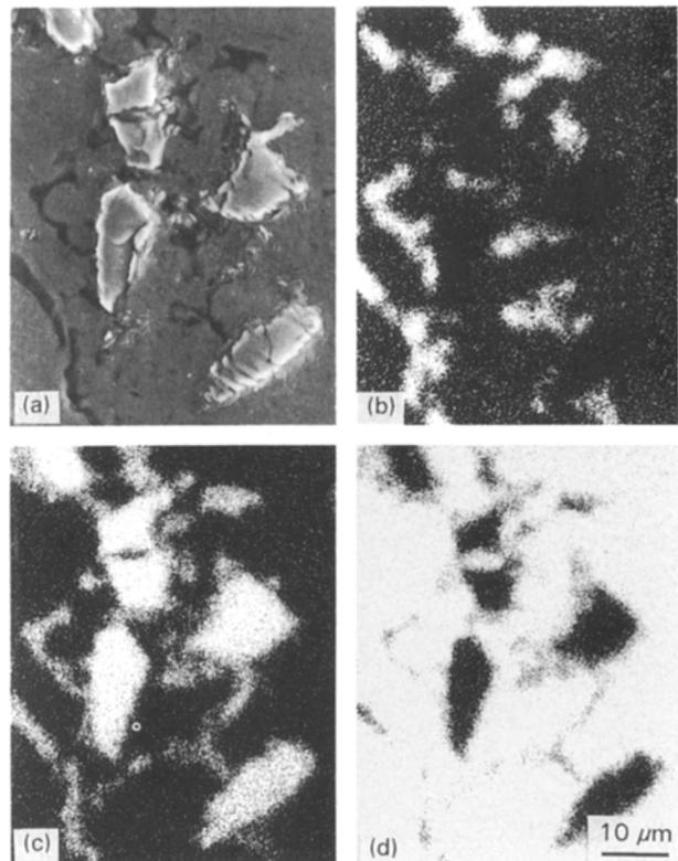
Figure 7 (a) Scanning electron micrograph, and X-ray images of (b) Mg, (c) Si and (d) Al for a cross-section of a SiC (20 μm)/Al-5.0% Mg composite.
