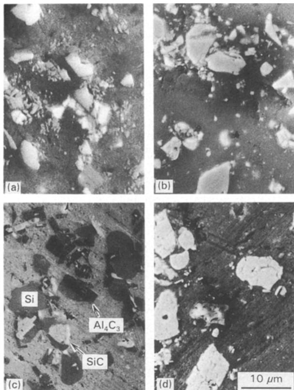
Figure 10 Scanning electron micrographs of (a), (c) SiC (3.0 μm)/Al and (b), (d) ZrC (2.4 μm)/Al composites. (a), (b) Without, and (c), (d) with holding at elevated temperature.
