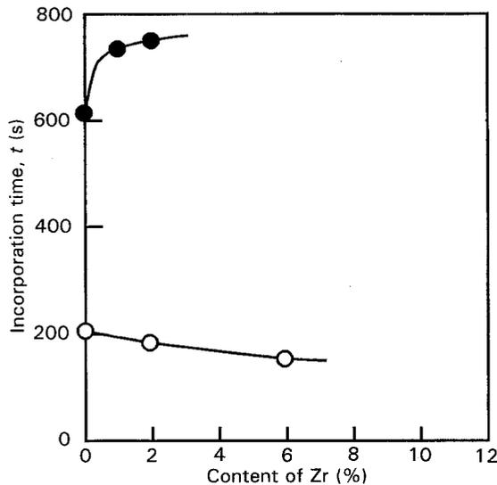
Figure 5 The effect of Zr alloying on the incorporation time of SiC (20 μm) and ZrC (2.4 μm) particles into liquid aluminium at 1023 K: (●) ZrC/Al-Zr, and (○) SiC/Al-Zr.
