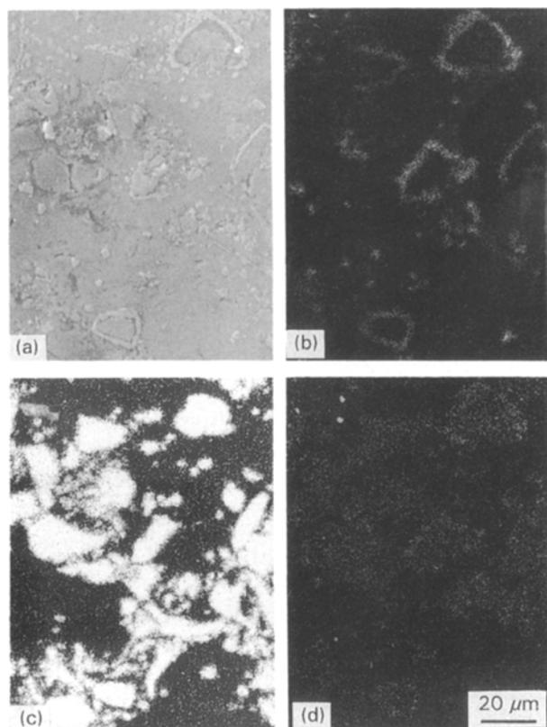
Figure 8 (a) Scanning electron micrograph, and X-ray images of (b) Ti, (c) Si and (d) C for a cross-section of a SiC (20  $\mu\text{m}$ )/Al–1.0%Ti composite.
