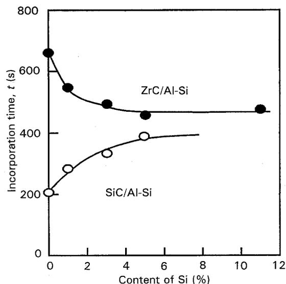
Figure 3 The effect of Si alloying on the incorporation time of SiC (20  $\mu\text{m}$ ) and ZrC (2.4  $\mu\text{m}$ ) particles into liquid aluminium, at 1023 K.
