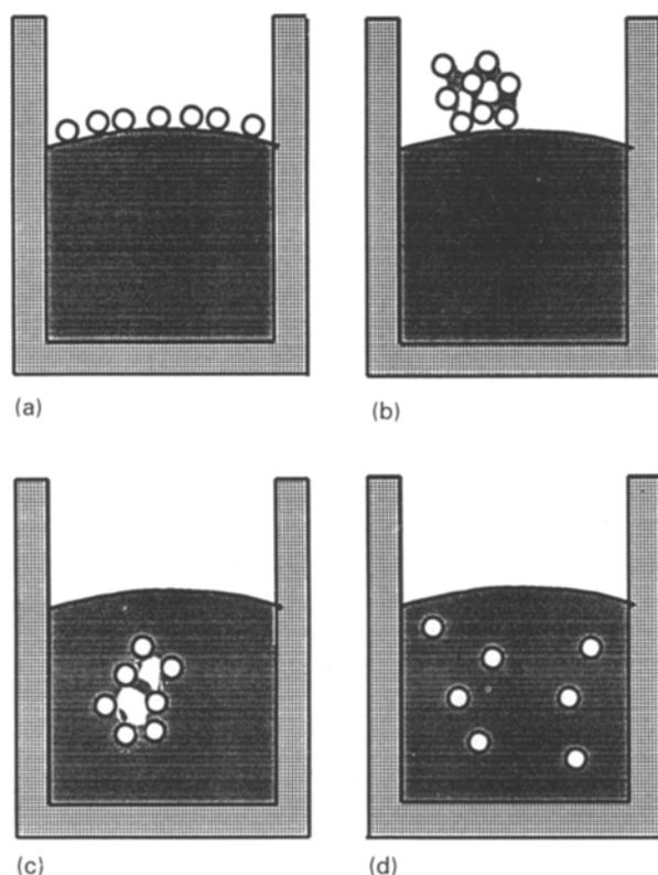
Figure 2 Schematic drawings of the incorporation process of ceramic particles into liquid aluminium: (a) addition of particles, (b) lumping, (c) incorporation, and (d) dispersion.
