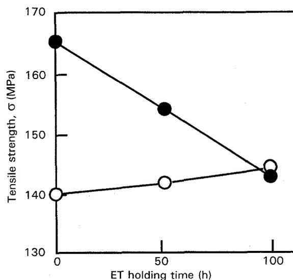
Figure 9 Changes in the SiC (20  $\mu\text{m}$ ), and the ZrC (2.4  $\mu\text{m}$ )/Al composites' strengths caused by the elevated-temperature (ET) holding at 803 K: (●) SiC/Al, and (○) ZrC/Al.
