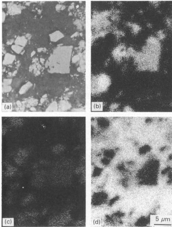
Figure 4 (a) Scanning electron micrograph; and X-ray images of (b) Si, (c) Zr and (d) Al for a cross-section of a ZrC (2.4 μm)/Al-11.6% Si composite.
