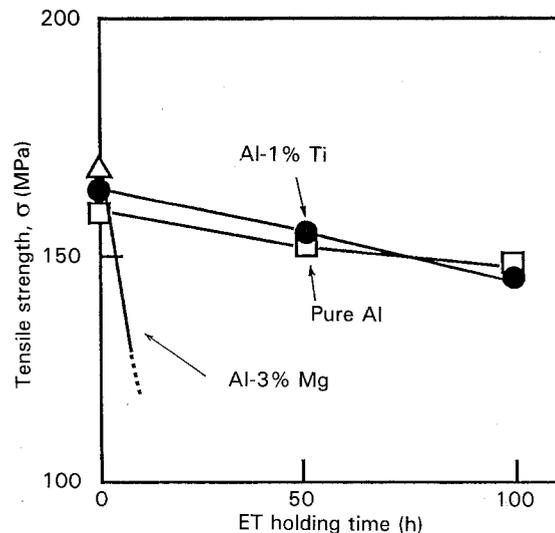
Figure 12 Changes in the SiC (3.0 μm)/Al alloy composite's strength caused by the elevated temperature holding at 803 K.
