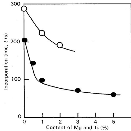
Figure 6 The effects of Mg and Ti alloying on the incorporation time of SiC (20 μm) particles into liquid aluminium at 1023 K: (●) SiC/Al-Mg and (○) SiC/Al-10Sn-Ti.
