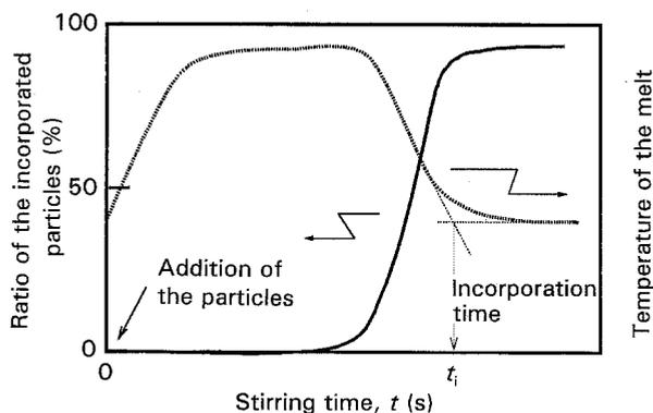
Figure 1 Typical relation between the ratio of incorporated particles, temperature of the liquid phase and the stirring time.
